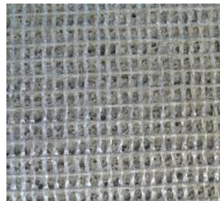
Cross hatched woven synthetic secondary backing
